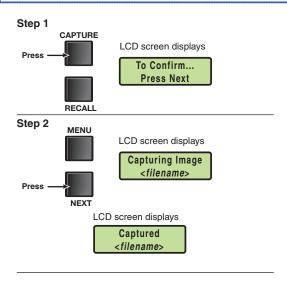
Figure 13. Sequence for Capturing an Image
